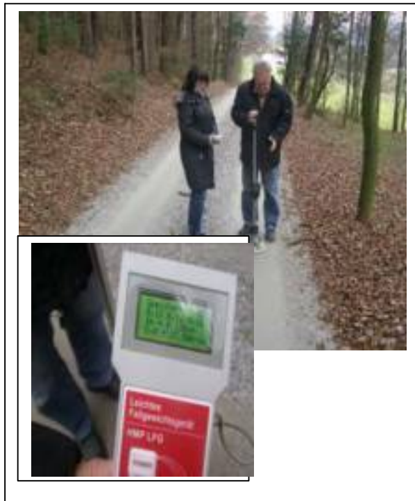
Field test bearing capacity
