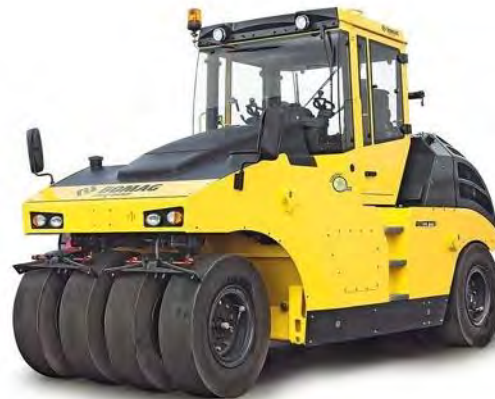
Pneumatic roller for spot compaction, weight at least 20 tons
